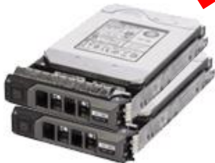
Worker node's local RAID 1 SSD hard drives for OS and /tmp
